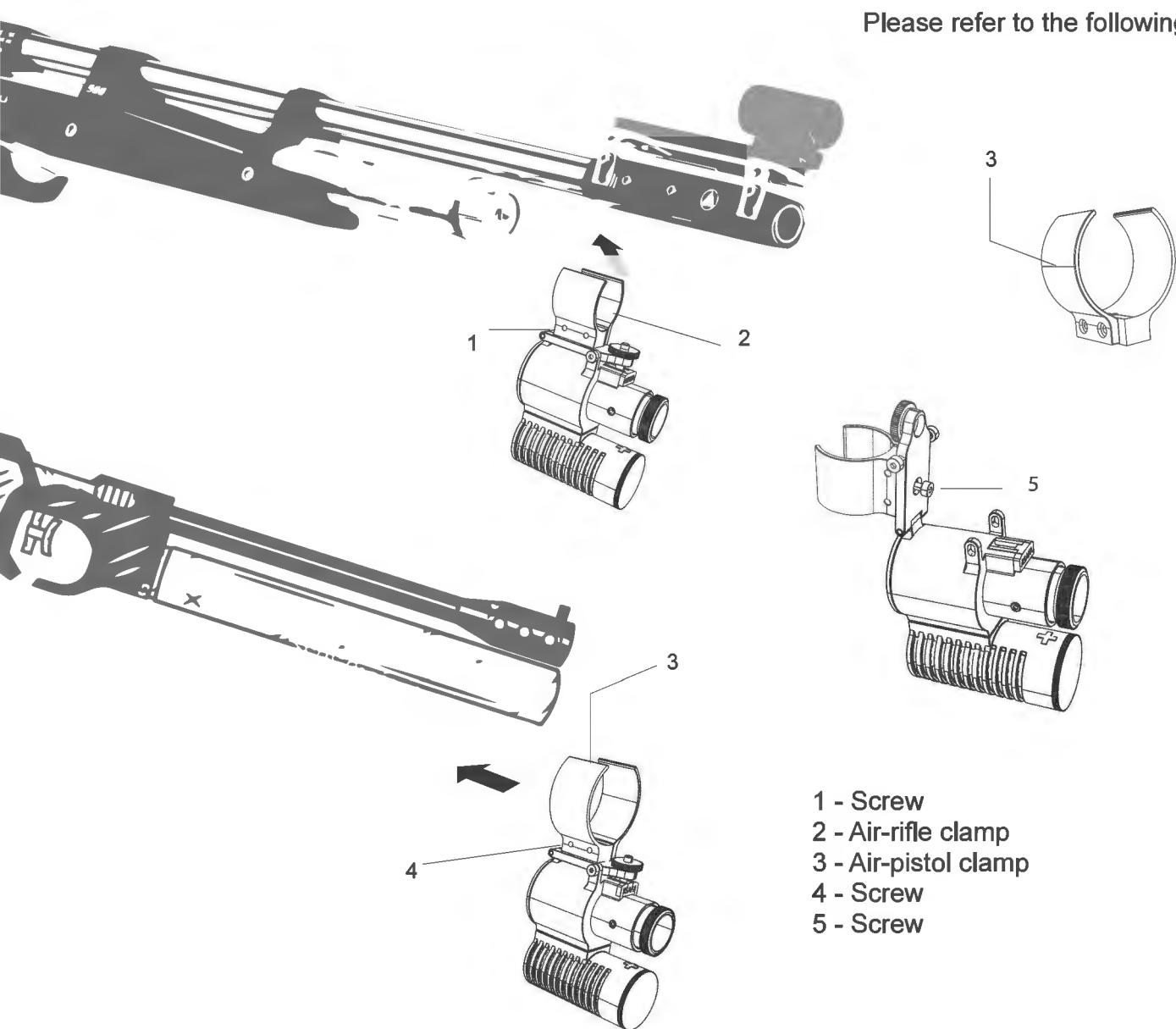
Loosen screw #1, and mount the air-rifle clamp #2 in the air-rifle tube. Fix screw #1.
